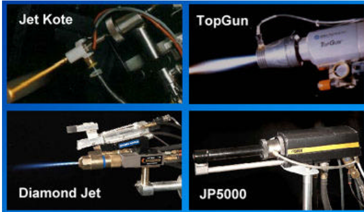
Figure 3 The most common commercially available HVOF spraysystems
